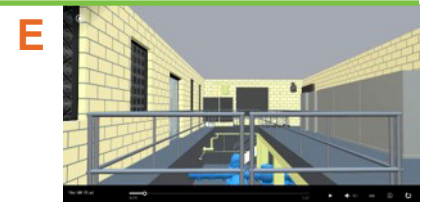
E New railing to meet OSHA standards and improved access in front of electrical panels.
