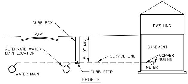
NOTE: COPPER TUBING IS REQUIRED THROUGH THE FOUNDATION WALL AND ON BOTH SIDES OF THE METER. THE COPPER TUBING SHALL BE SECURED ON BOTH SIDES OF WHERE THE METER IS TO BE LOCATED. METER IS TO BE PLUMBED HORIZONTALLY WITH APPROPRIATE CLEARANCE ON ALL SIDES. SPACING WILL VARY DEPENDING ON METER SIZE. CONTACT E.C.W.A. METER SHOP FOR QUESTIONS REGARDING SPACING REQUIREMENTS.
